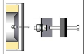
Screw the fixing screw tight.
