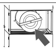
Unhook the cartridge holder from the cartridge guides.
